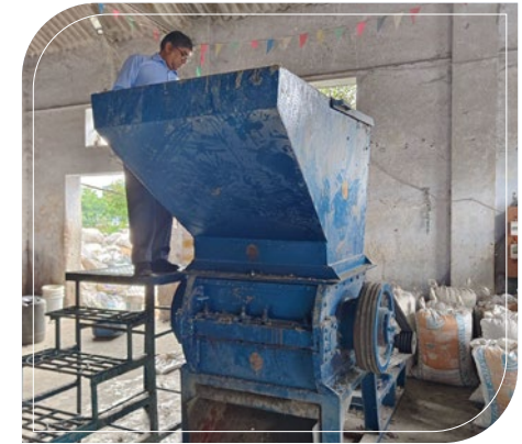
Shredding machine at the site
